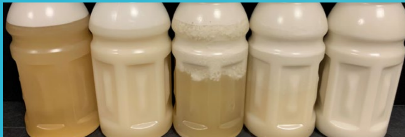
BOTTLE 1-4 : Infant formula samples with different degrees of product separation. Without the appropriate food additives, infant formula separates into lipid- (top) and water-soluble (bottom) fractions
